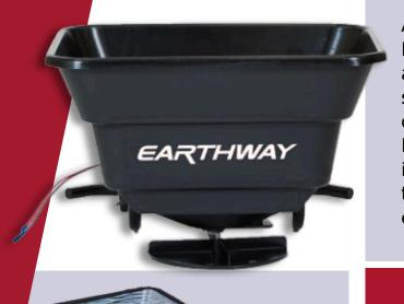
A great additional tool for your ATV. The M20 has an 36 kg rustproof poly hopper and even spread 3-hole drop shut-off system to ensure even uniform coverage of fertilizer, seed, chemicals, and more. Equipped with a 12-volt motor located inside the hopper, and housed in a thermal-plastic case, the M20 is engineered for performance and long life.
